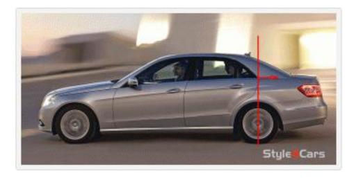
The car in the image is RWD. As explained in the previous rule, that kind of cars has the front wheels closer to the corners than the FWD. In other words, the entire cockpit is pulled back to make place for the longitudinally placed engine. So, the C pillar, which marks the rear end of the cockpit, begins over the axis of the rear wheels. In the FWD the cockpit is moved a little bit forward, in relation with the RWD car, so the C pillar usually is centred in its base over the rear wheel axle.
